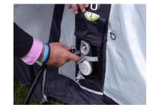
7. Repeat steps five and six with the other AirFrame Tube. Then replace the caps and cover with the Velcro sleeve neatly to ensure the valve is covered.
